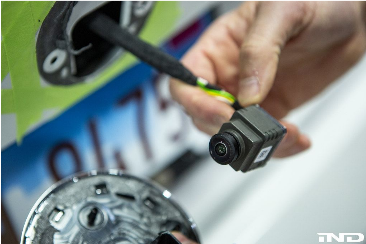
Figure 6 — The factory roundel is now fully separated from the camera assembly. Set the factory roundel aside; the camera will be transferred into the new IND roundel.
