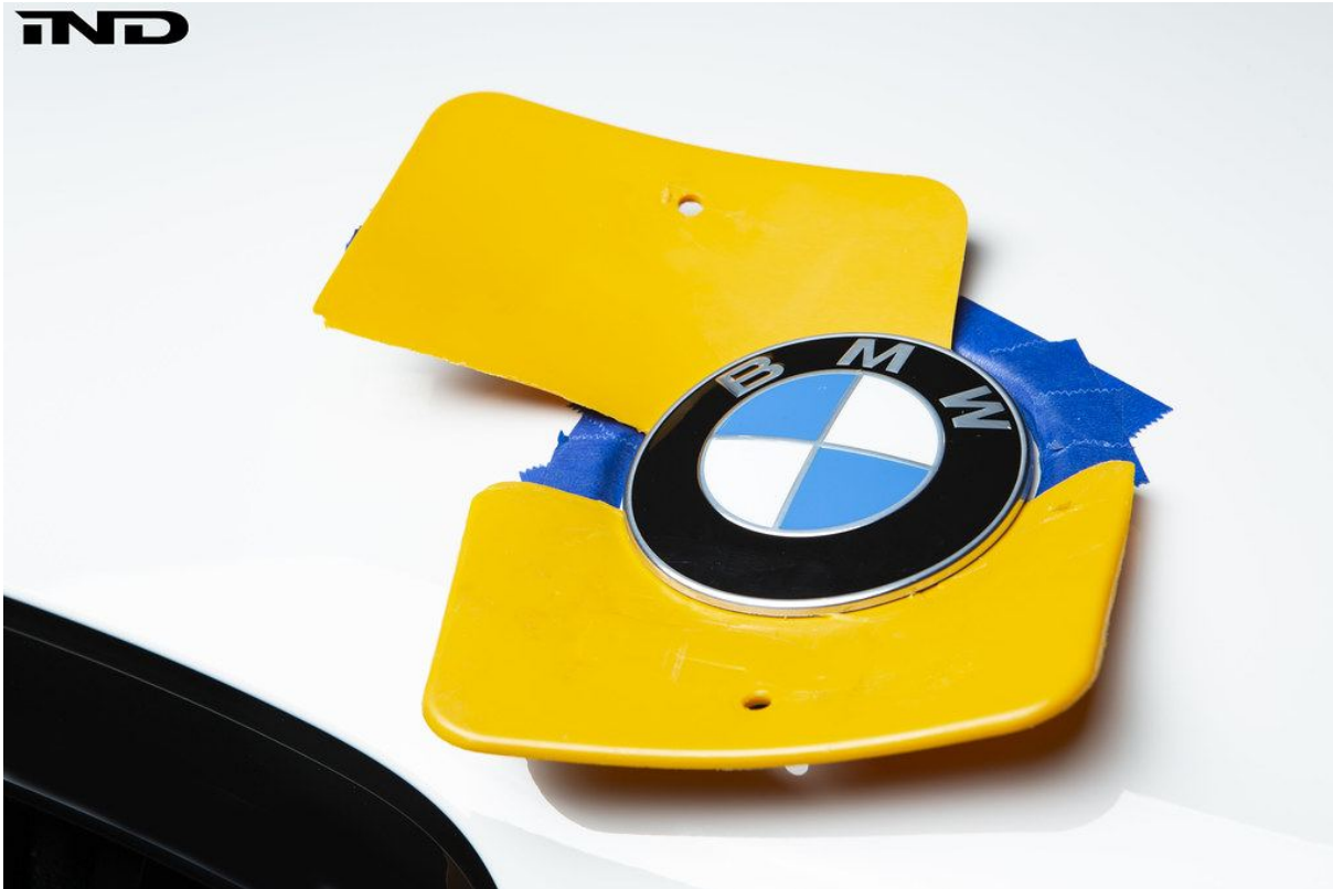
Figure 2 — The IND bondo spreader is worked behind the factory roundel to gradually break the adhesive bond around the perimeter.
