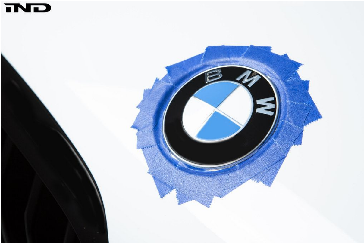
Figure 1 — Painter's tape applied around the perimeter of the factory front roundel. The tape provides a buffer between the paint and the spreader during removal.
