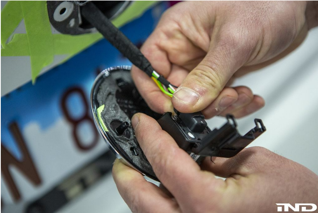
Figure 5 — The reverse camera assembly is gently lifted out of the factory roundel housing.
