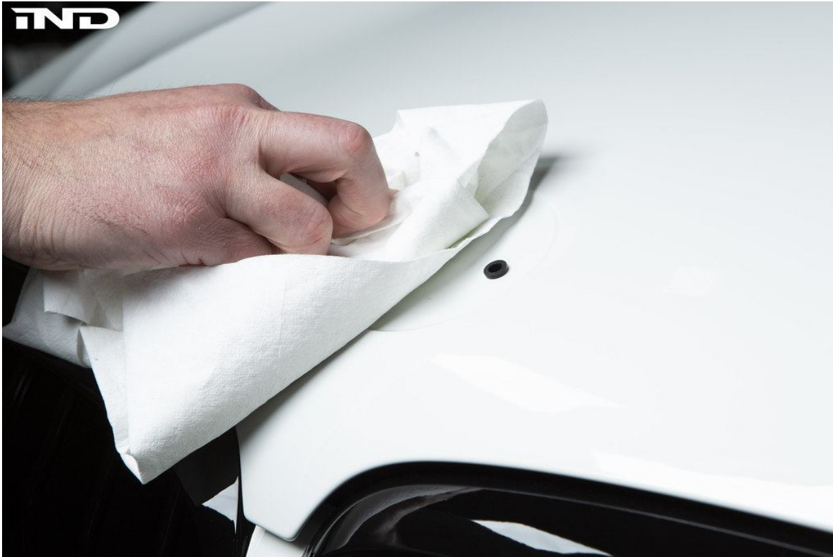
Figure 4 — Isopropyl alcohol applied with a microfiber towel removes all residual adhesive and prepares the mounting surface for the new roundel.
