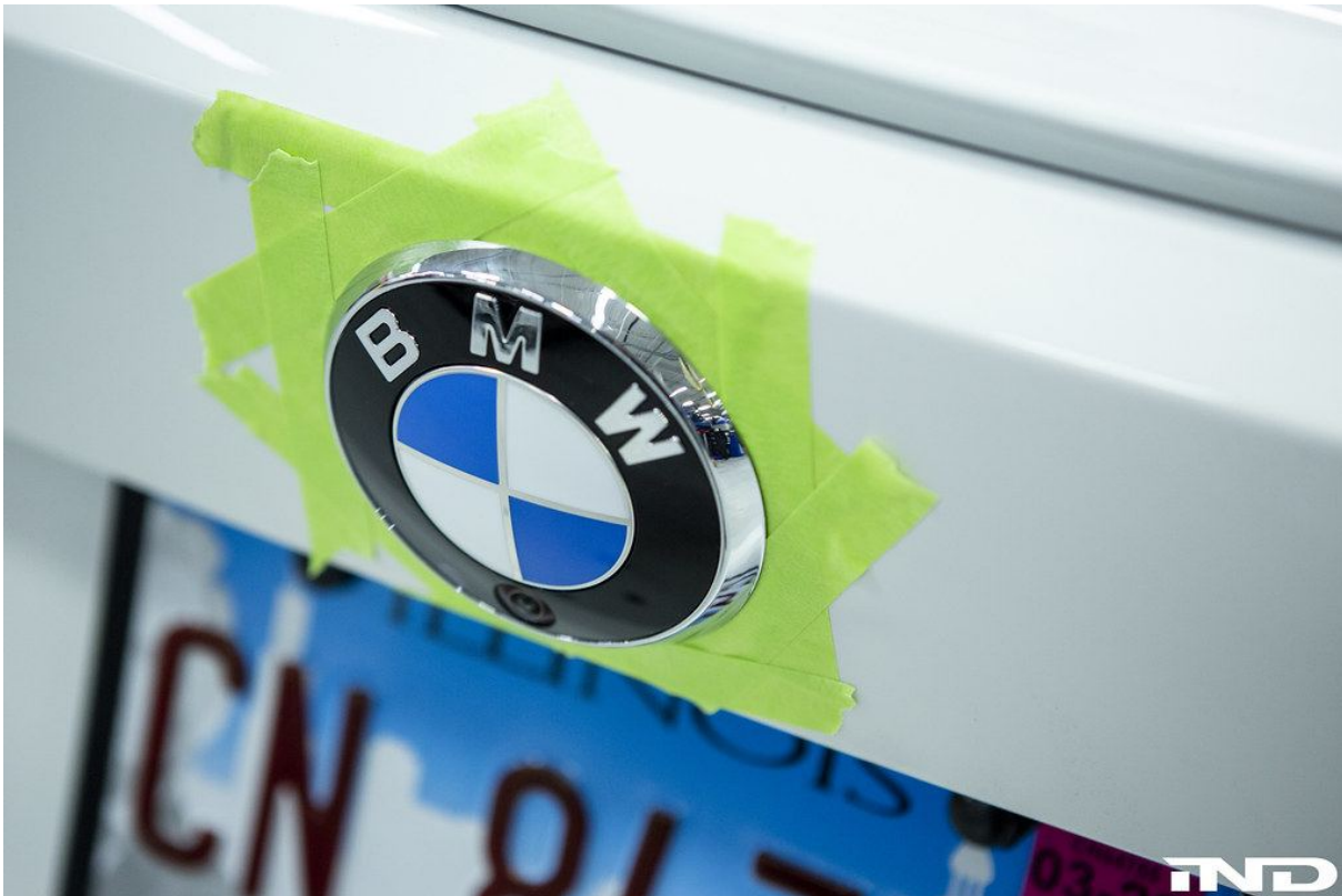
Figure 1 — Painter's tape applied around the perimeter of the rear roundel before any tools are introduced.
