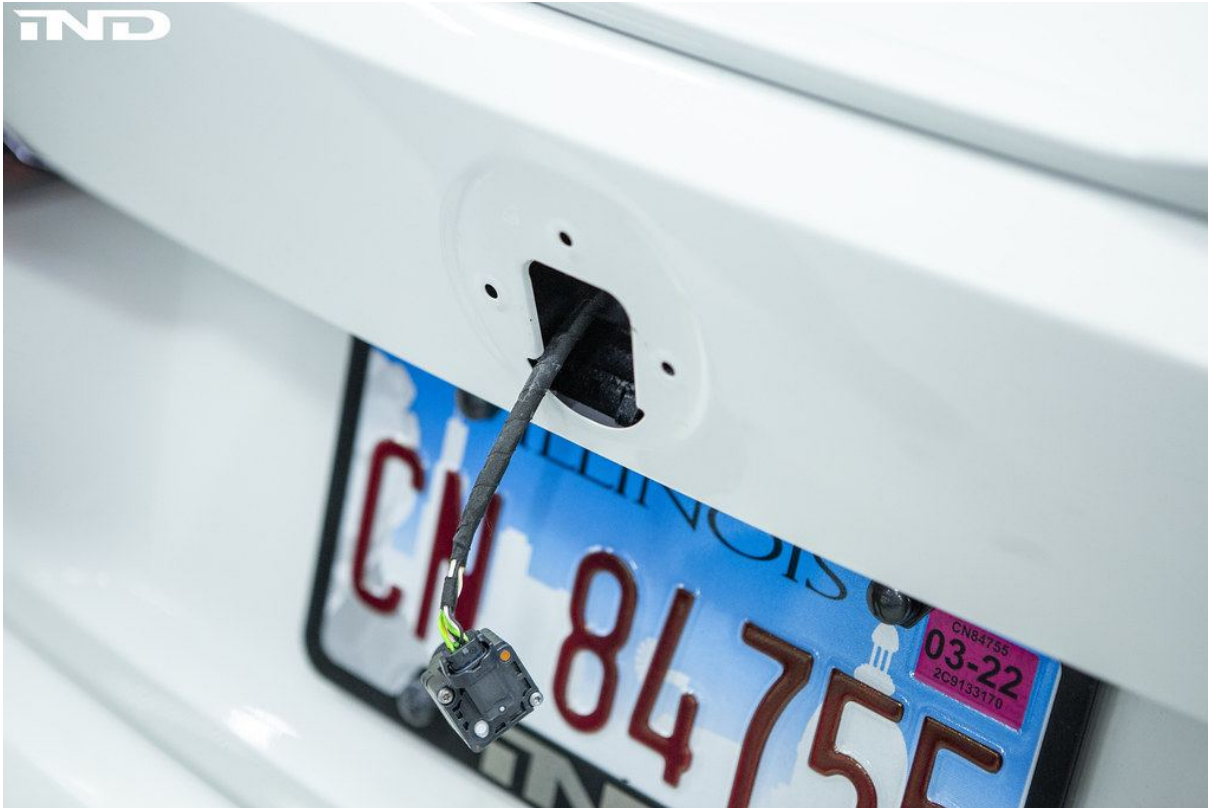
Figure 8 — The trunk mounting surface fully cleaned and prepared. The surface should be free of adhesive residue and contaminants.
