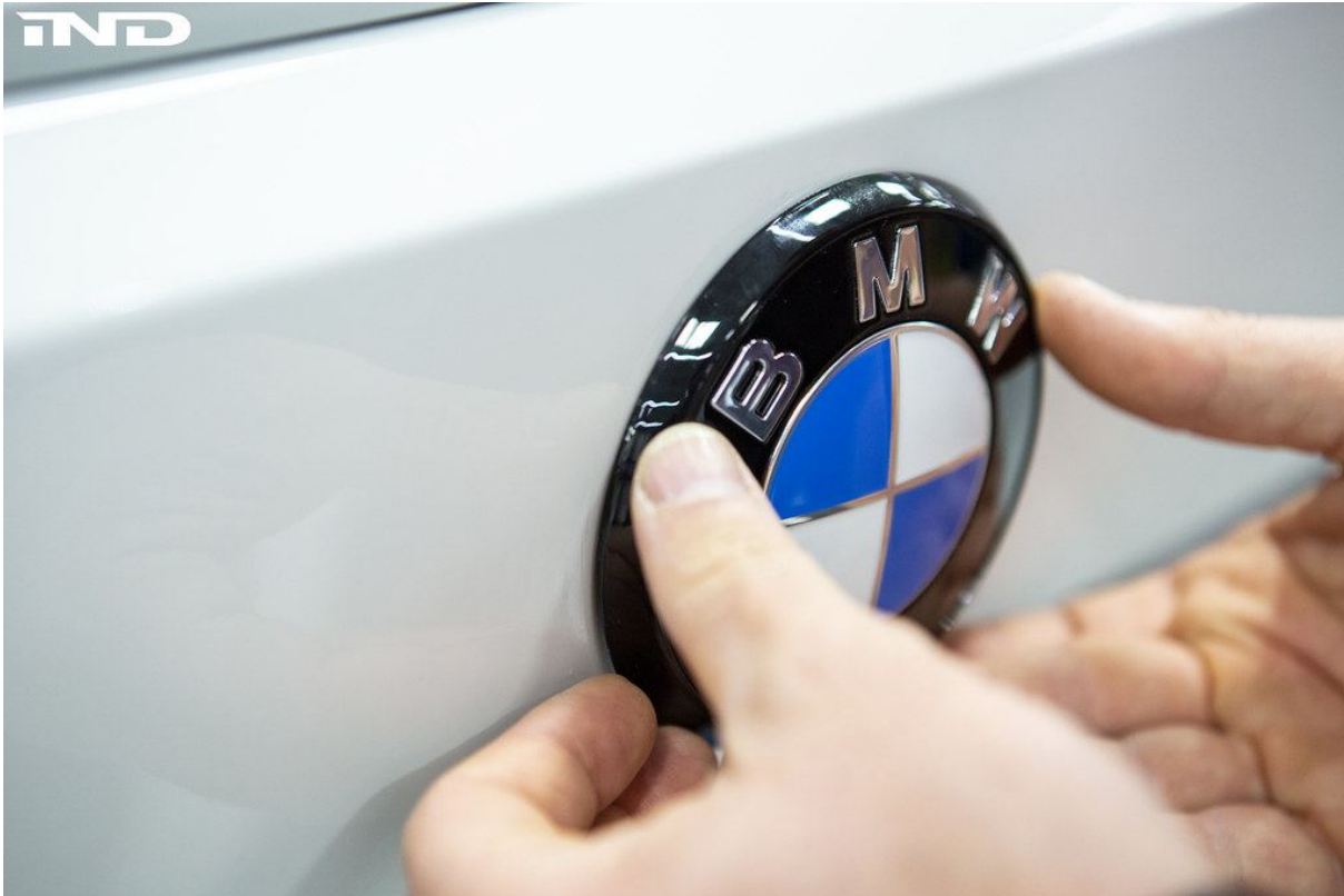
Figure 11 — The new IND painted rear roundel pressed firmly into the factory mounting location. Apply uniform pressure across the entire face to seat the adhesive.
