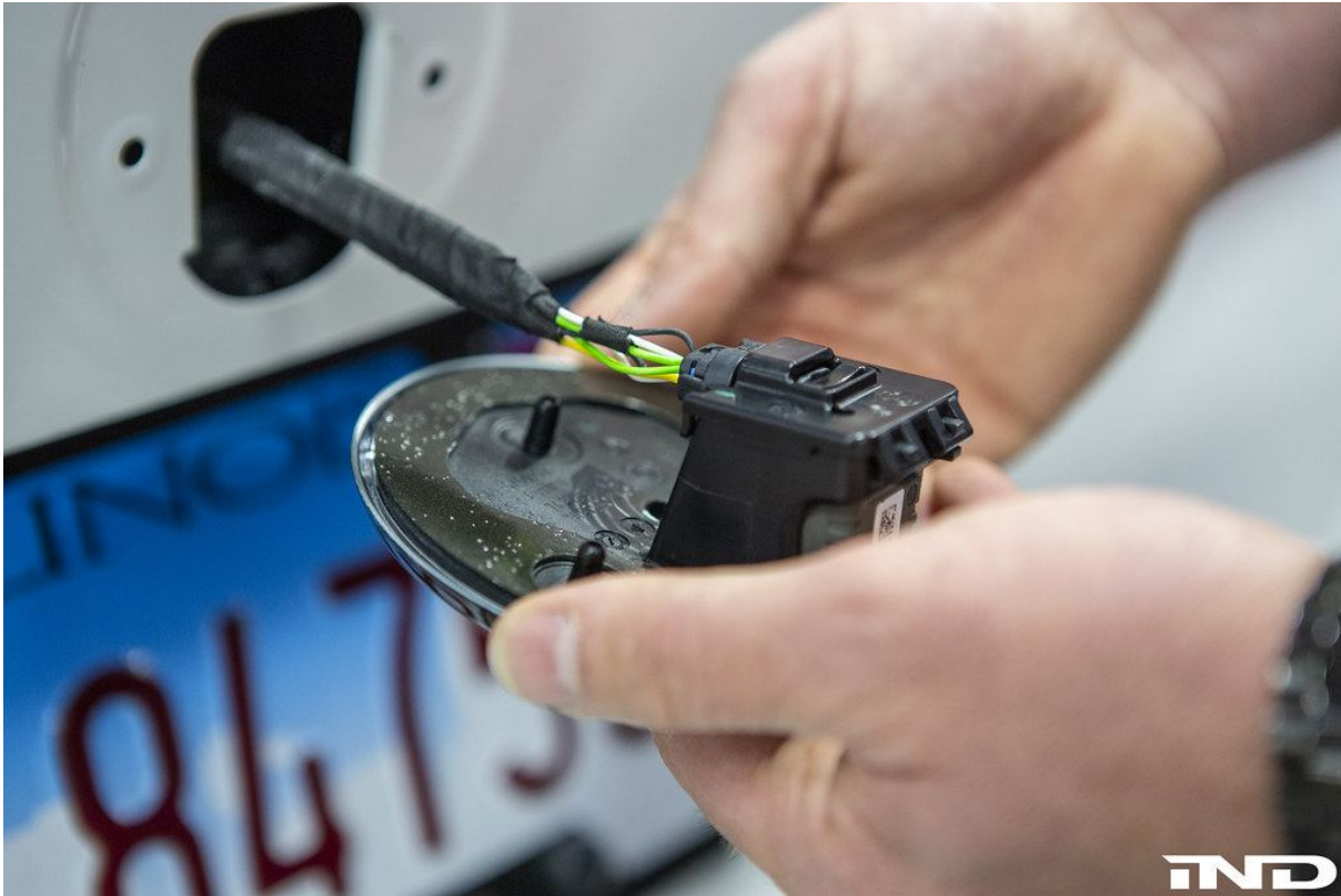
Figure 10 — The reverse camera assembly transferred into the new IND painted roundel. Both retaining clips on the housing cover must fully engage.
