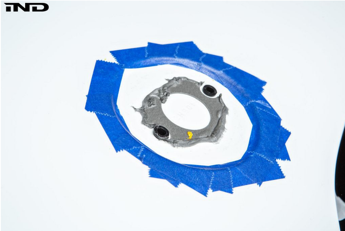
Figure 3 — The factory roundel after removal. Note the residual foam tape and adhesive on the body panel that must be cleaned away before the new roundel is installed.
