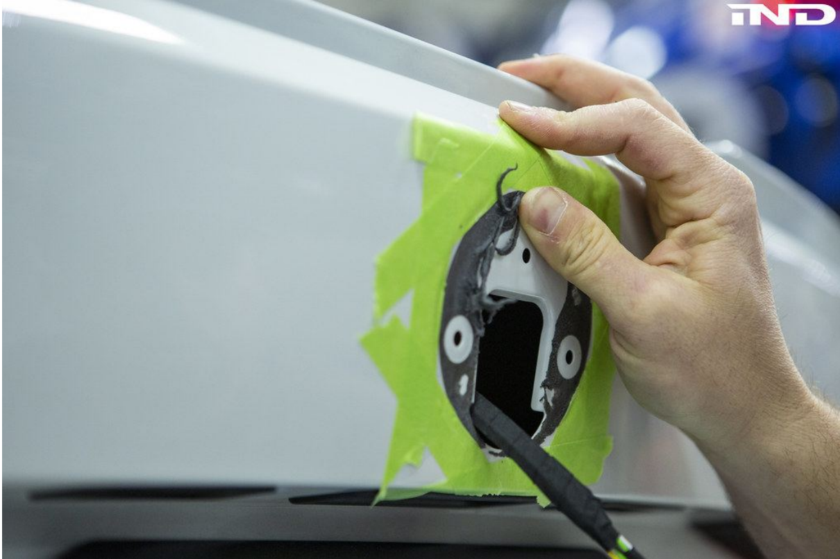
Figure 7 — Rubbing the foam tape with your thumb gently rolls the adhesive away from the trunk panel without scratching the paint.
