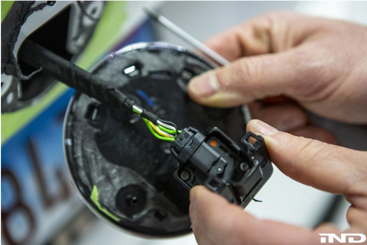
Figure 4 — The camera housing on the back of the factory roundel. Two small retaining clips secure the cover and must be released to access the camera.
