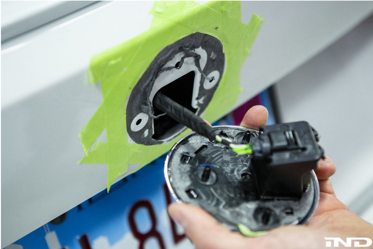
Figure 3 — The rear roundel lifted from the trunk panel with the reverse camera assembly still attached. Note the camera harness remains connected to the vehicle.
