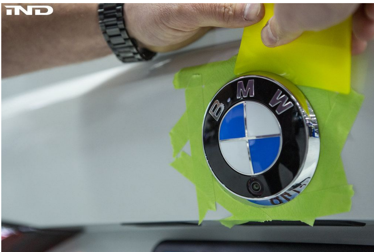
Figure 2 — The IND bondo spreader works behind the rear roundel to release the adhesive. The roundel remains tethered to the vehicle by the camera harness behind it.
