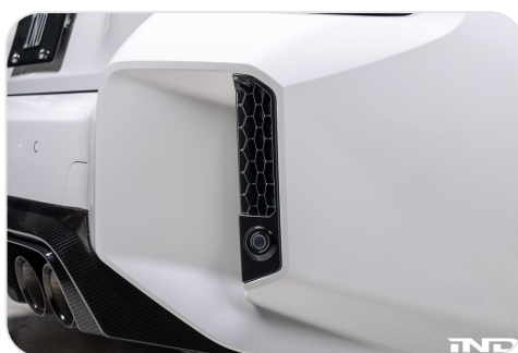
Completed Acexxon Honeycomb insert with the factory PDC sensor retained.
