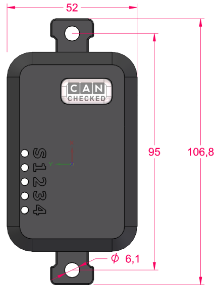
Figure 2 - Mounting receiver (All dimensions in mm)
